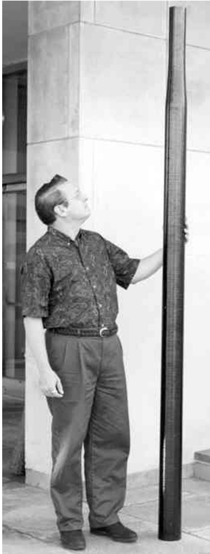
Fig. 22 Braided GE90 carbon-PMR vent tube
