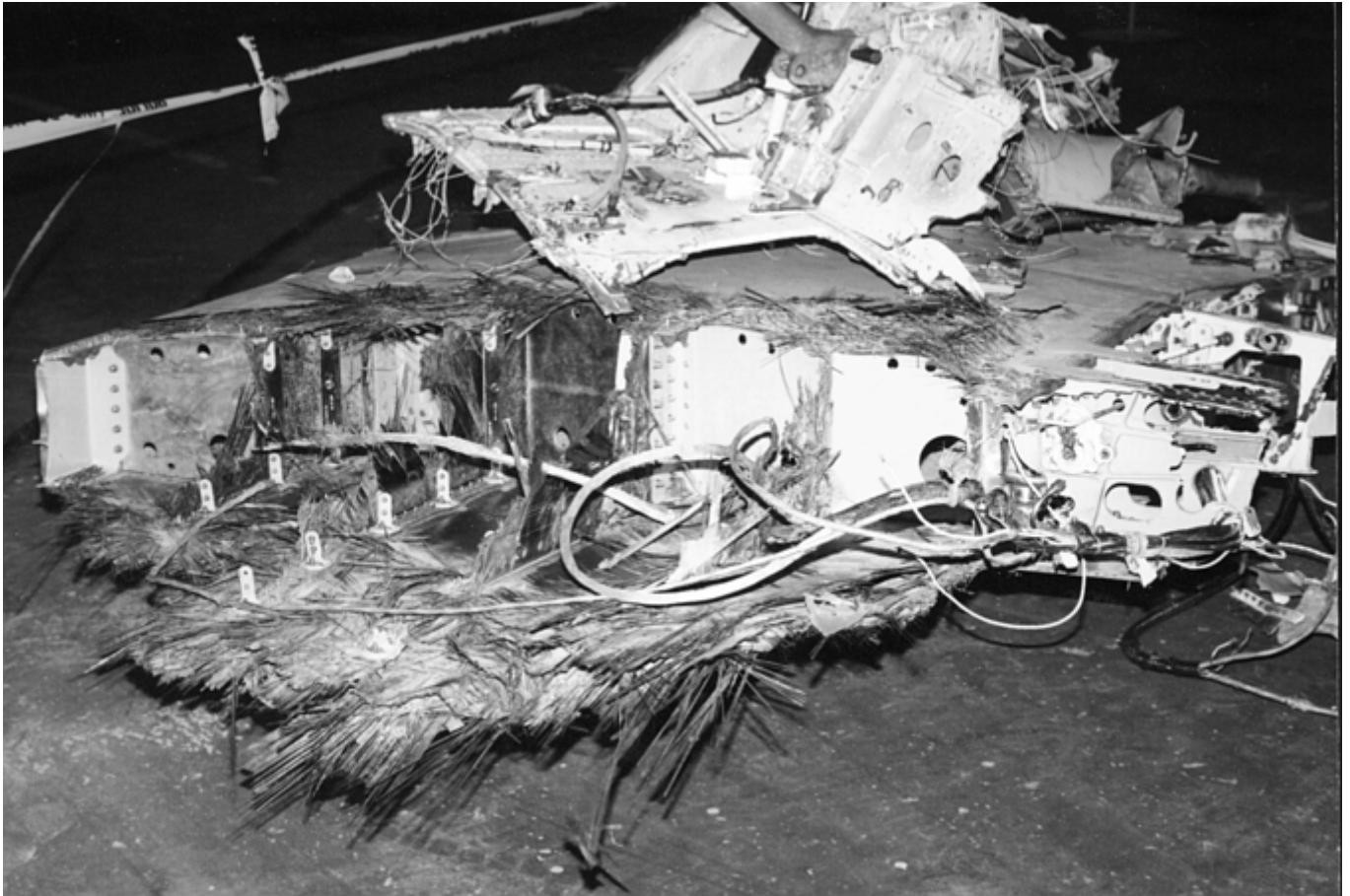
Fig. 2 Flexural failure of a graphite-epoxy wing box. \sim 0.03\times
