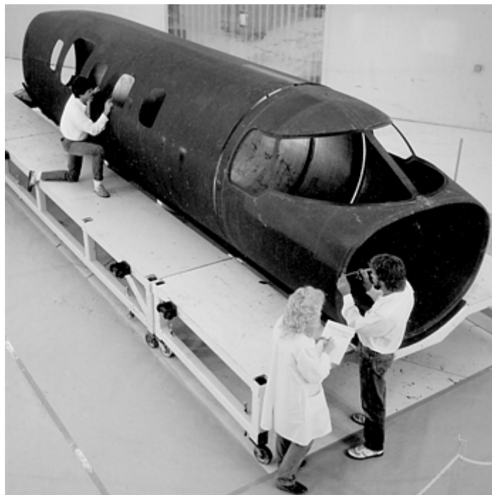
Fig. 10 Beech Starship filament-wound fuselage. Courtesy of Fibertek Division of Alcoa/TRE, Inc.
