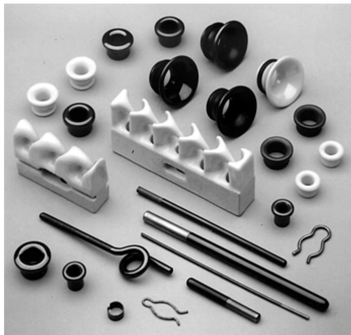
Fig. 22 Typical pigtail and ceramic guides. Courtesy of Texkimp, Ltd.
