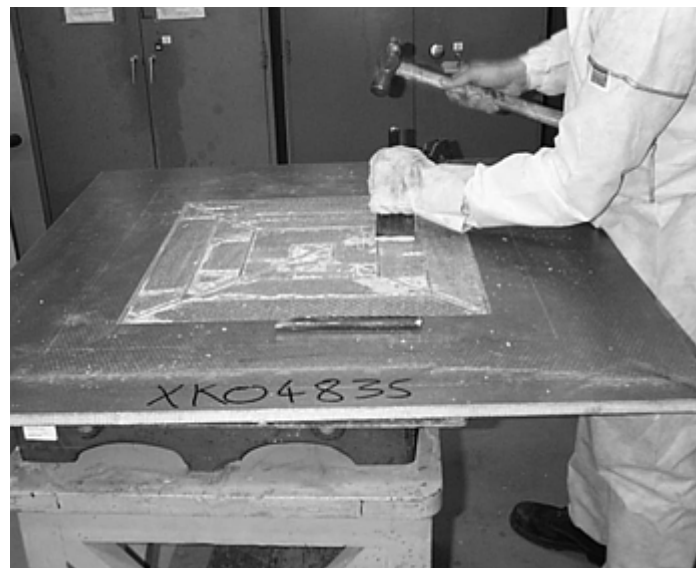
Fig. 10 Mechanical extraction of damage to form a step profile
