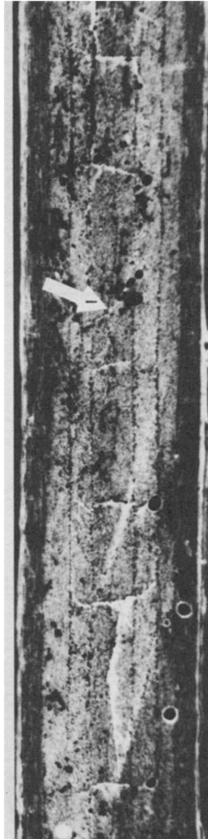
Fig. 9 Edge replica of graphite-epoxy specimen
