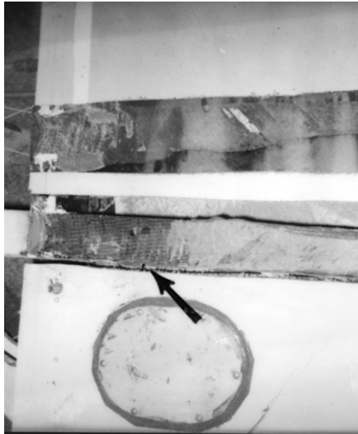
Fig. 8 Mating fracture surfaces of an adhesively bonded wing skin and wing spar. ~0.2×
