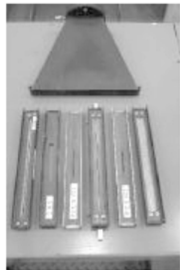
Fig. 32 Example of an in-motion radiography facility showing (a) the facility, (b) a close-up of the source robot, and (c) the collimator and slits
