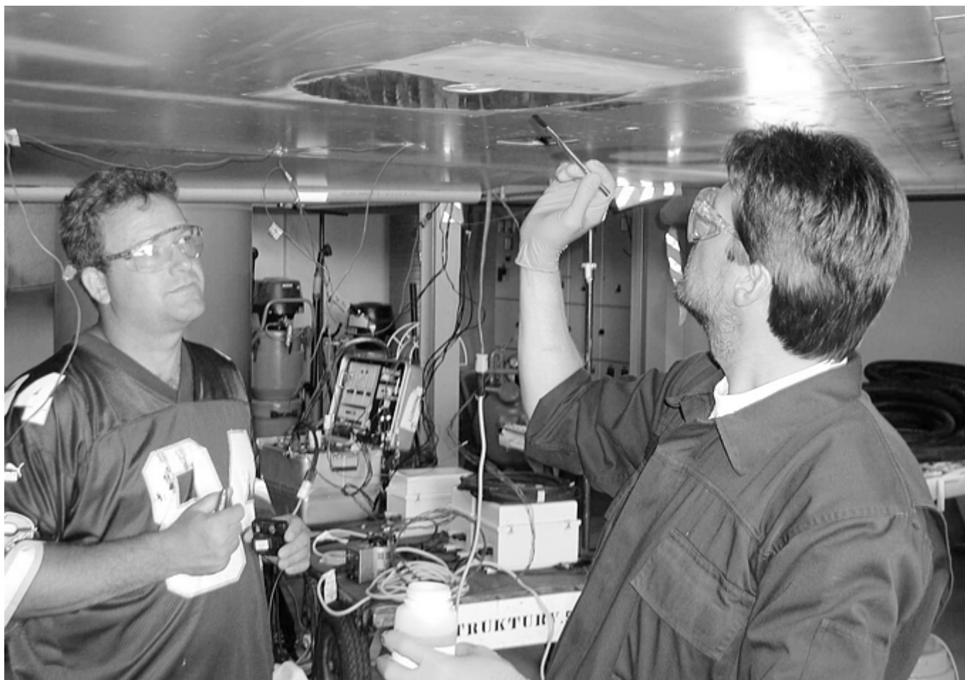
Fig. 2 Application of silane coupling agent (GBS surface preparation) during a F-16 aircraft repair
