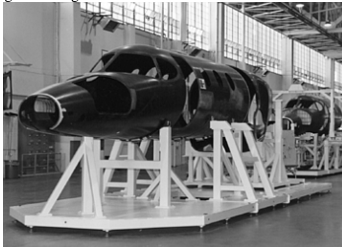
Fig. 4 Raytheon Premier I fuselage manufactured by fiber placement
