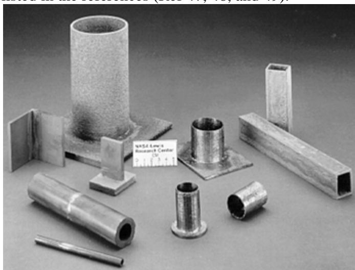
Fig. 3 Illustrations of various SiC and SiC composites joined using melt infiltration, a reaction-forming process to make various components. Courtesy of M. Singh, NASA Glenn Research Center
