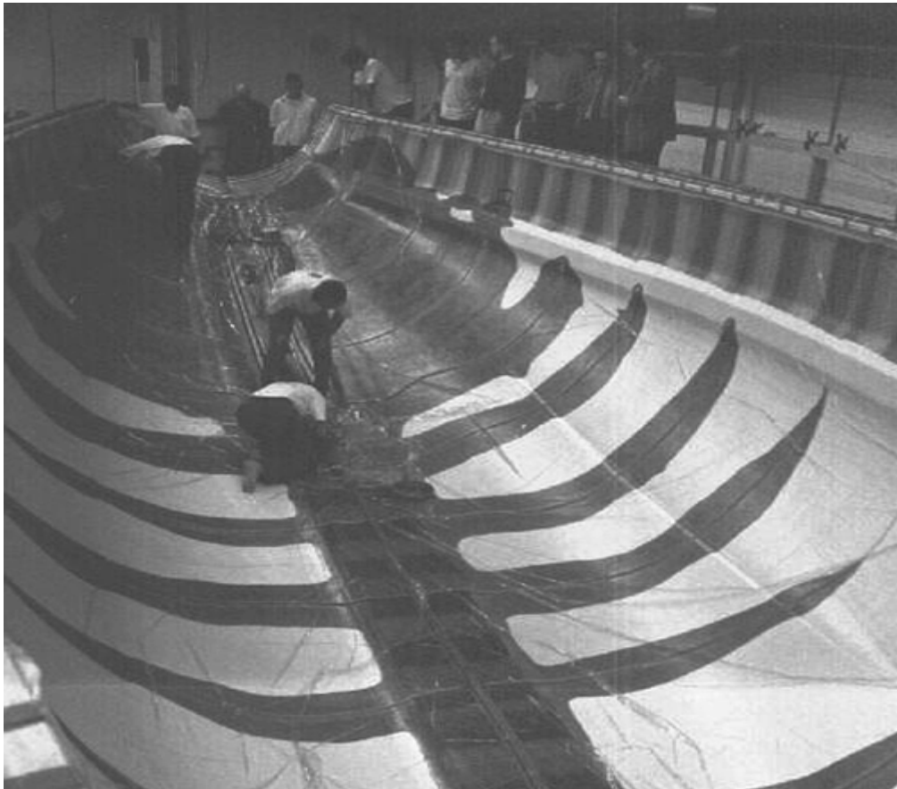
Fig. 3 Contest 55 sailing yacht with hull manufactured by vacuum infusion. Courtesy of Conyplex Shipyard, Medemblik, the Netherlands
