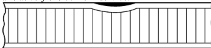
Fig. 2 Cosmetic repair using superficial nonstructural filler
