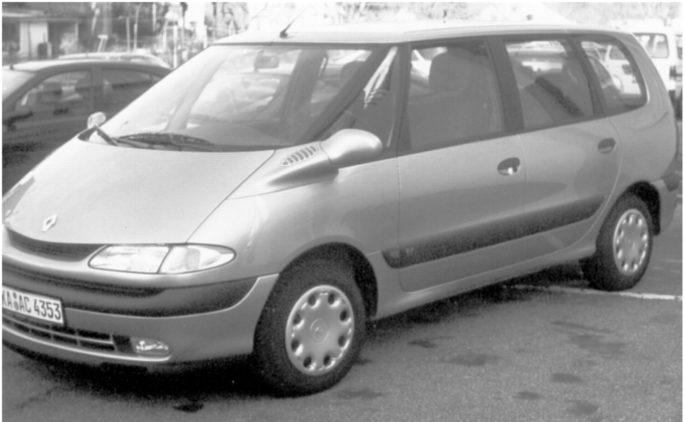
Fig. 39 Example of a minivan (Renault Espace) with exterior body panels made by SMC compressions molding
