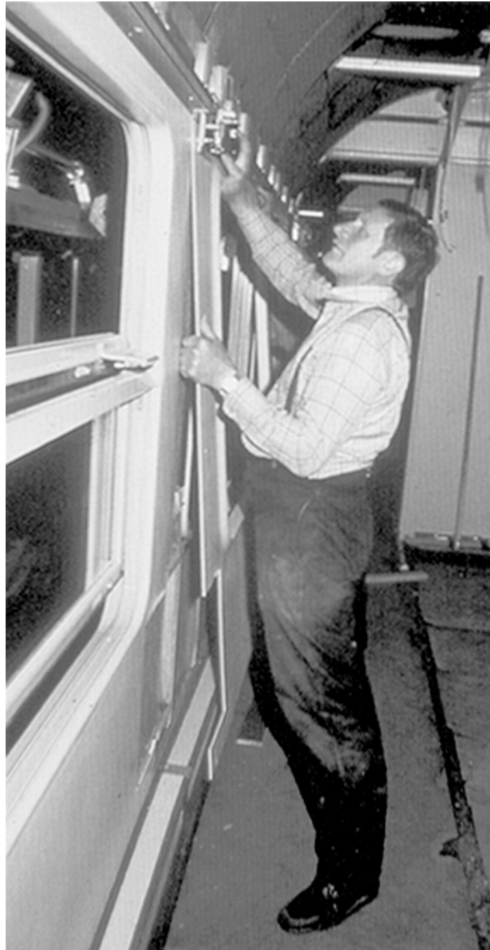
Fig. 42 Assembly of SMC compression-molded interior wall elements in passenger rail cars
