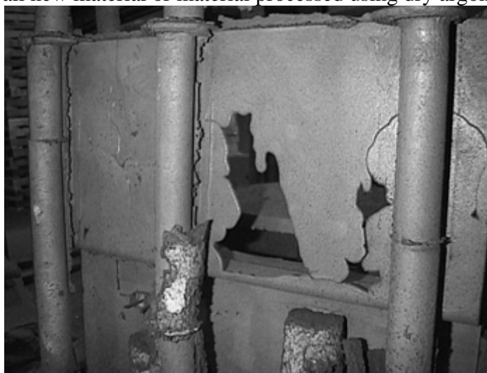
Fig. 1 Casting misrun due to low fluidity caused by presence of oxides in SiC/Al matrix MMC
