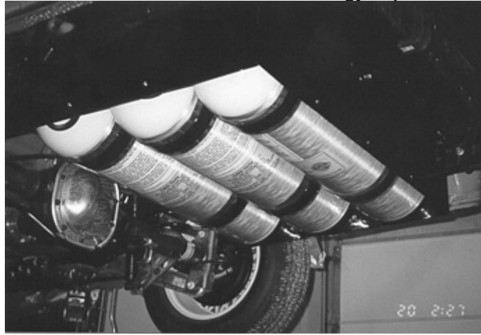
Fig. 11 Composite fuel storage tank. Reprinted by permission from the Society for the Advancement of Material and Process Engineering (SAMPE)
