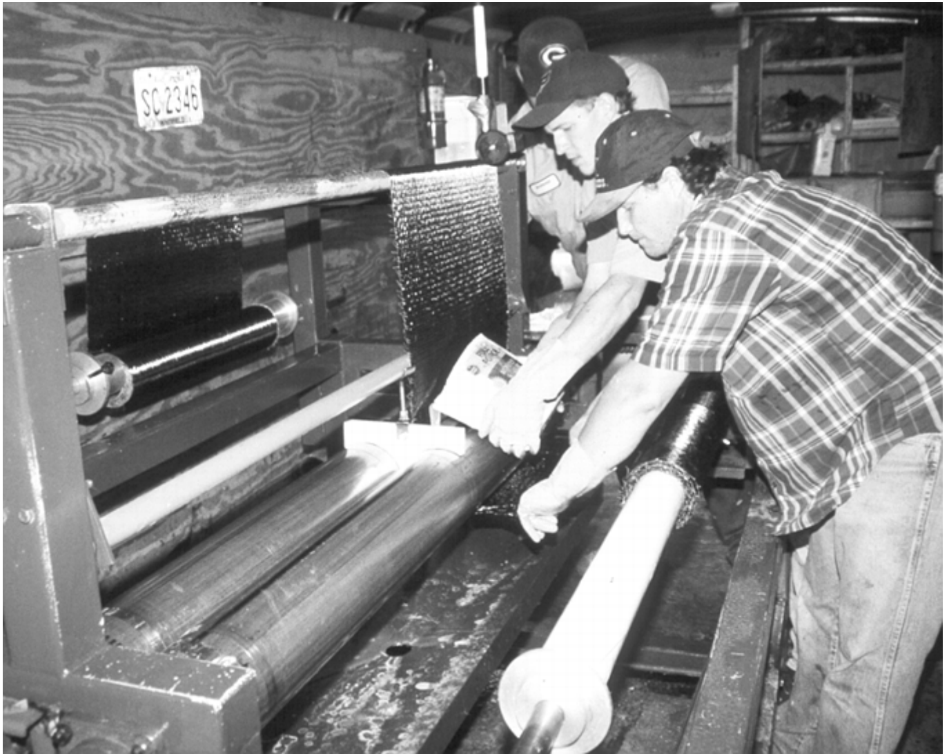
Fig. 3 Portable impregnator machine for field manufacture of fiber-reinforced composites
