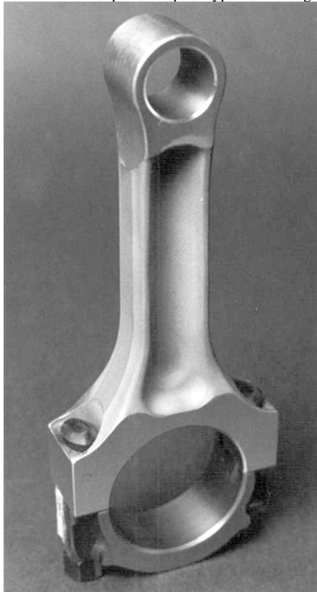
Fig. 3 Prototype aluminum MMC connecting rod
