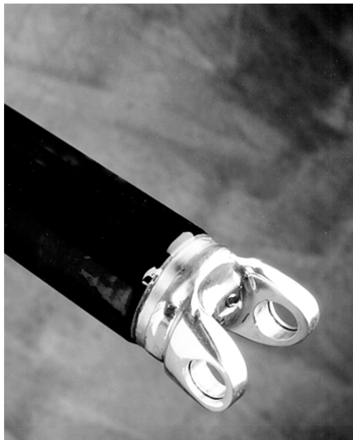
Fig. 23 Filament-wound composite driveshaft. Courtesy of ACPT
