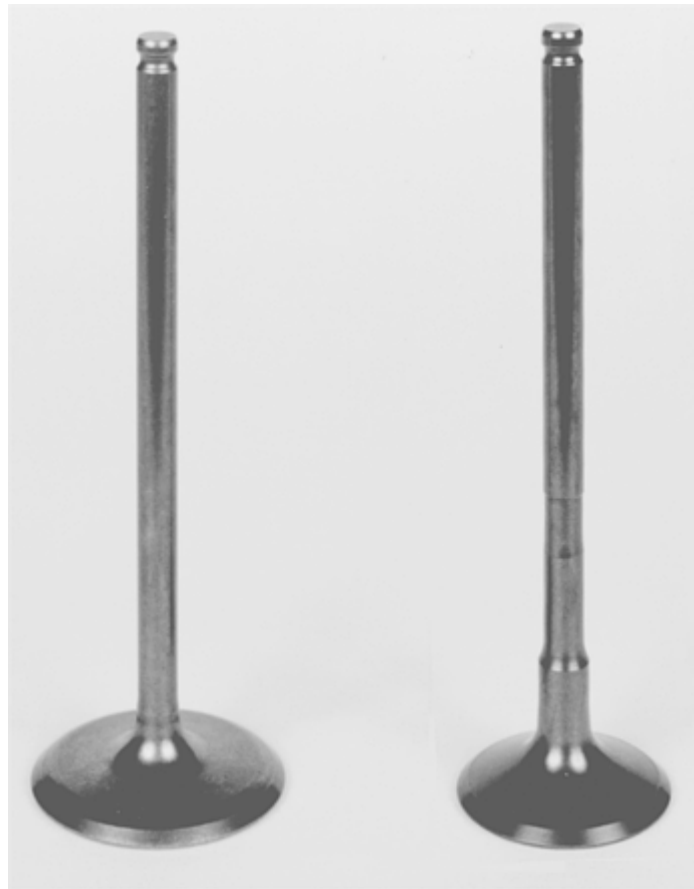
Fig. 2 Discontinuously reinforced titanium (DRTi) automotive valves for the Toyota Altezza. The valve on the left is an intake valve, and on the right is an exhaust valve. Courtesy of Toyota Central Research and Development Laboratories
