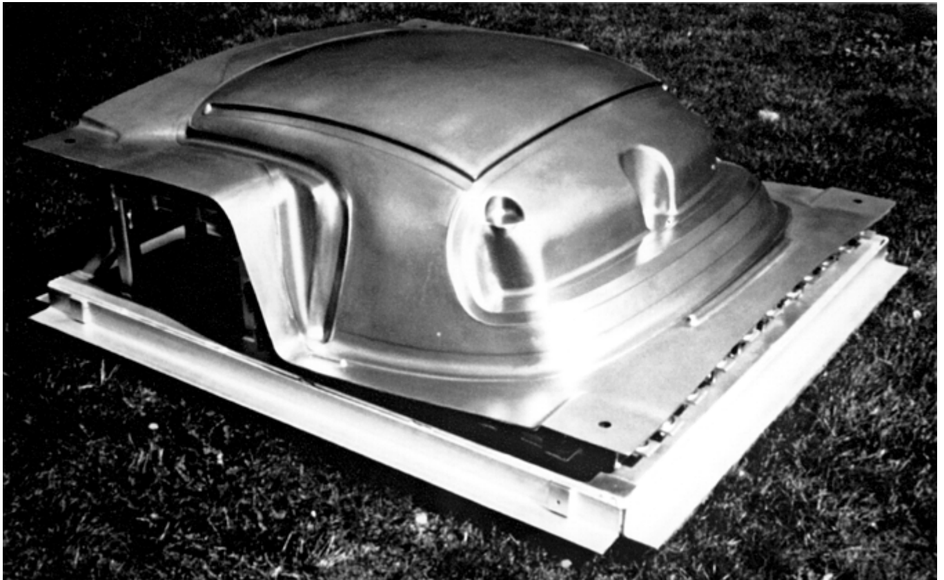
Fig. 3 Nickel shell male preform mold for composite auto roof
