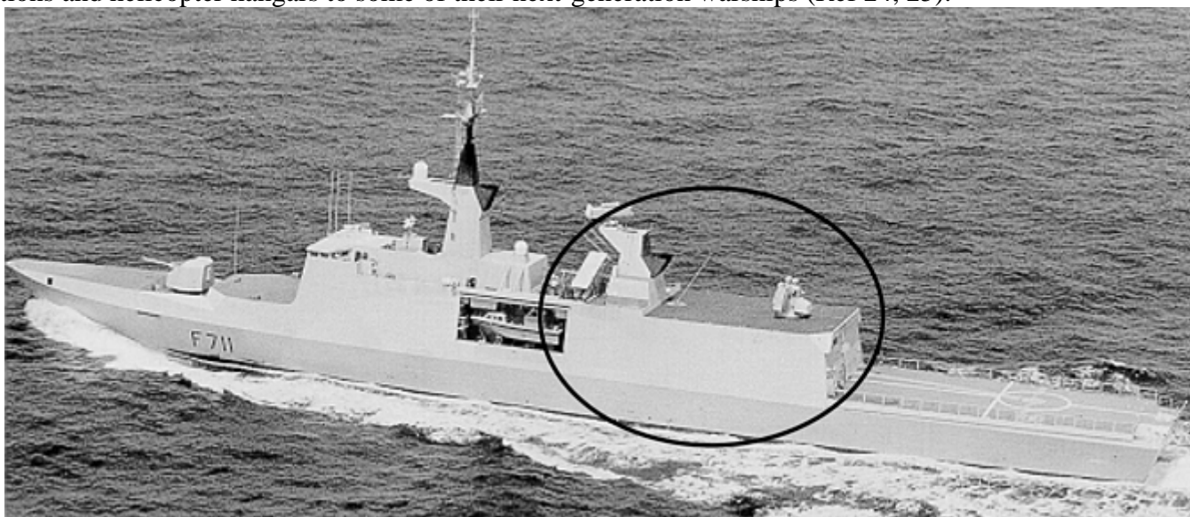
Fig. 4 La Fayette frigate with the composite superstructure section shown within the circled region
