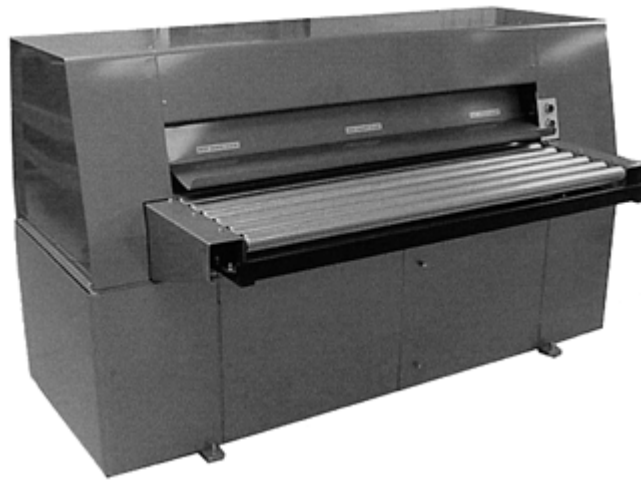
Fig. 4 Roller press with steel-rule dies. Courtesy of Century Design
