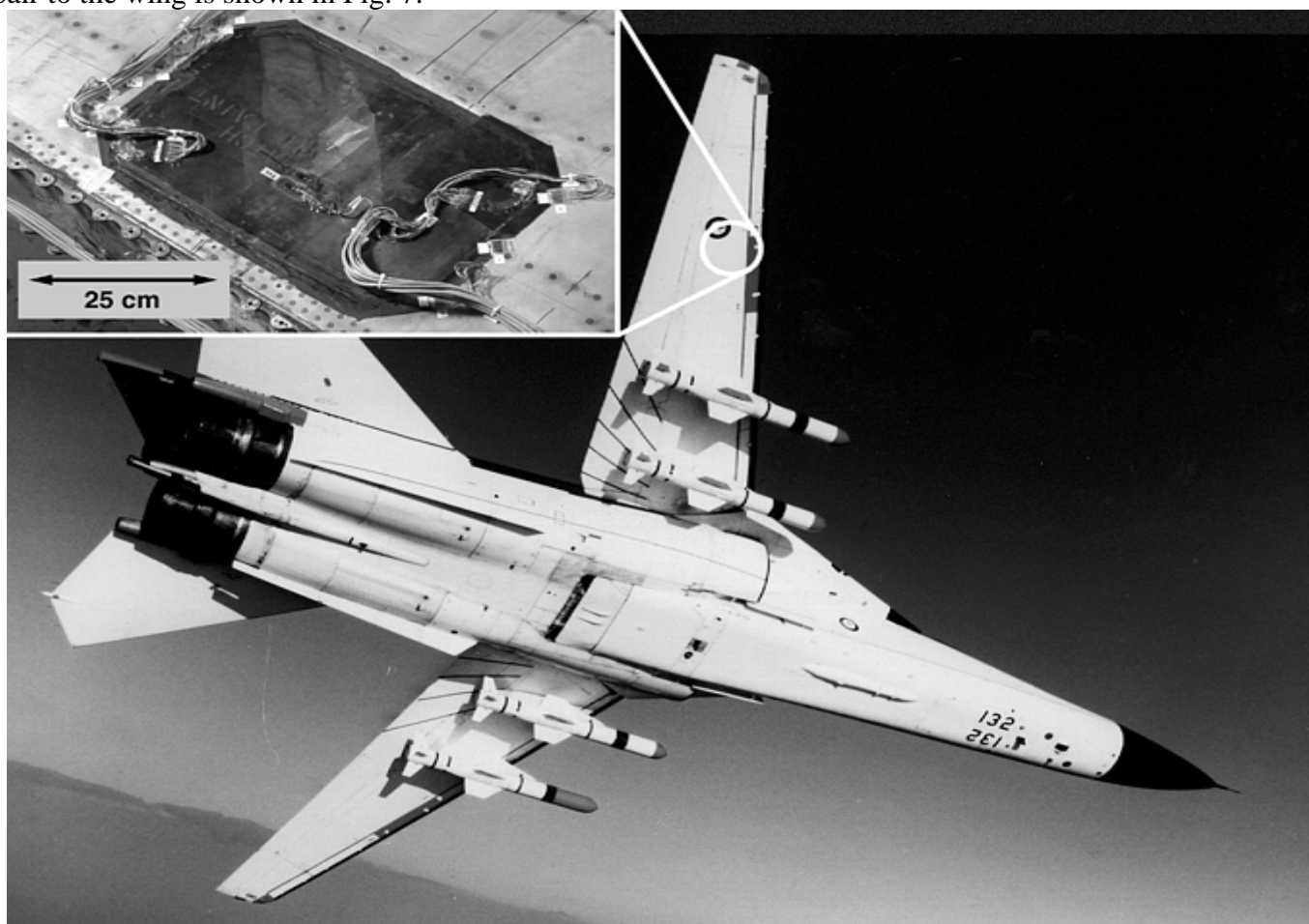
Fig. 7 Bonded composite repair to F-111 lower wing skin
