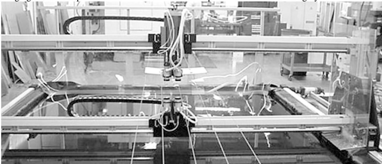
Fig. 3 Automated ultrasonic two-channel flat panel through-transmission system
