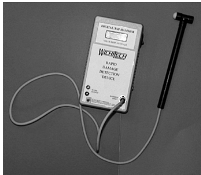
Fig. 14 Tap test for detecting delaminations between the composite layers or between the composite and concrete. Courtesy of Abaris Training
