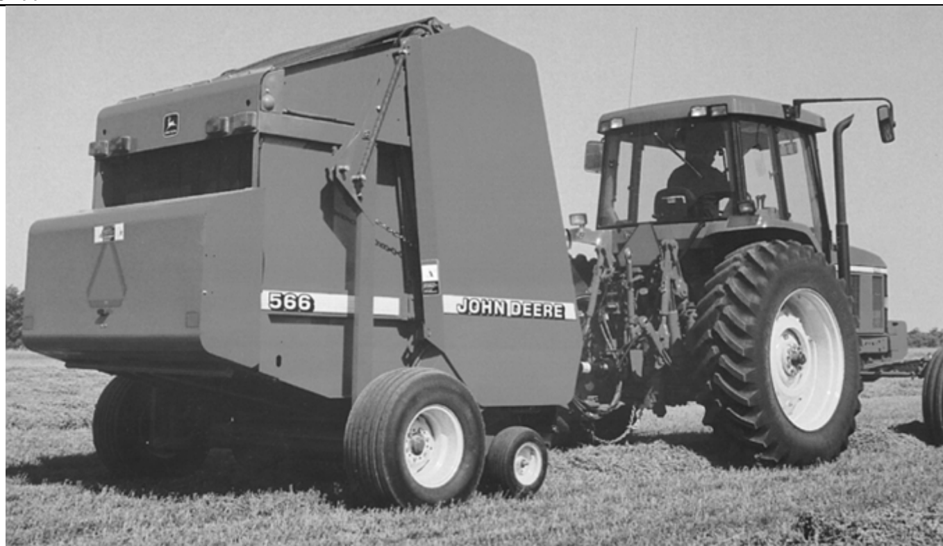
Fig. 8 Round hay baler. The 2.5 × 1 m (8 × 3 ft) panel containing the name “John Deere” was made from a soy- based resin. Courtesy of John Deere, Moline Illinois
