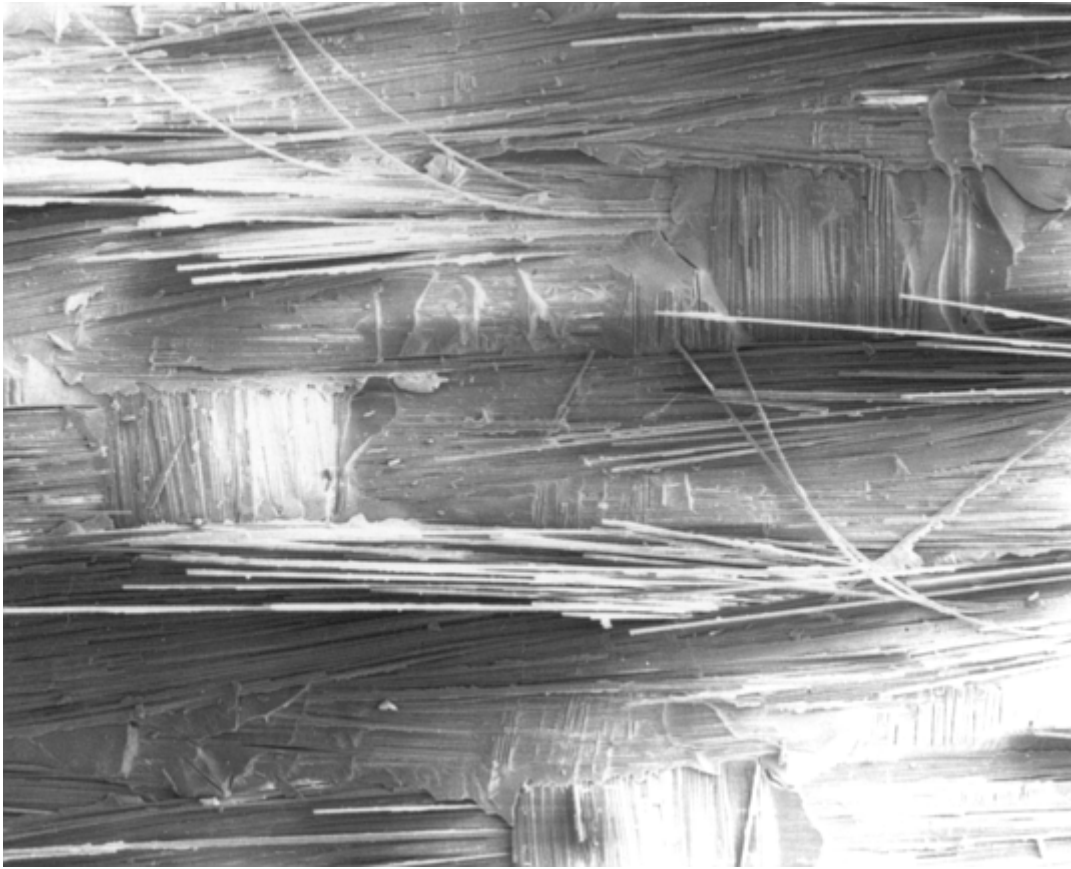
Fig. 12 Exposure of fiber splinters in a glass/polyimide laminate having inadequate resin content, following mode I tension loading of the specimen. 40×
