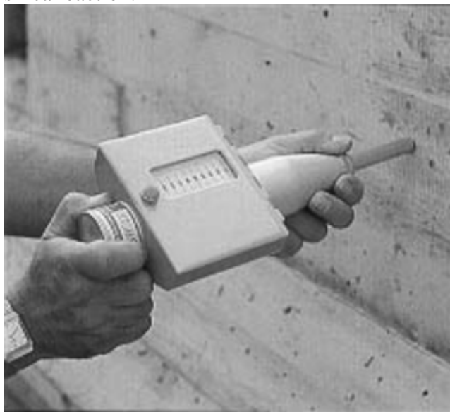
Fig. 1 Schmidt Hammer for evaluating concrete quality. Courtesy of PROCEQ SA
