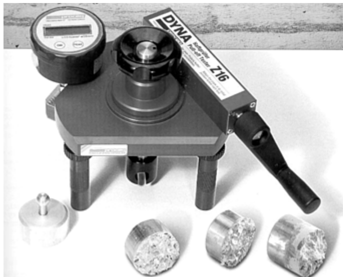
Fig. 17 Pull-off tester for measuring bond strength. Courtesy of PROCEQ SA
