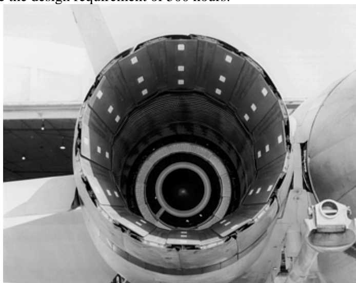
Fig. 9 Exhaust nozzle of an F414 engine on an F-18 E/F aircraft, showing the twelve sets of CMC flaps and seals. The white areas on the seals are a zirconia overcoat for mechanical fasteners. Over an order-of-magnitude increase in life has been obtained with the CMC flaps and seals.
