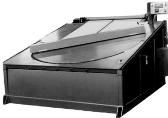
Fig. 3 Automatic angle-cutting prepreg sheeter. Courtesy of Century Design
