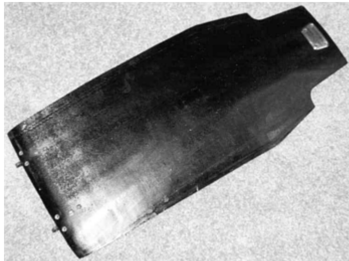
Fig. 10 Carbon-PMR General Electric (GE) F110-400 exhaust nozzle flap
