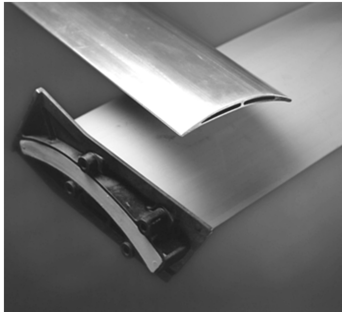
Fig. 5 Fan exit guide vane blank (top), showing the high quality of the as-extruded product and the double-hollow construction. Below is an assembled fan exit guide vane mounted in the endcap. This component is used in Pratt & Whitney 4084, 4090, and 4098 gas turbine engines. Component dimensions are provided in the text. Courtesy of DWA Aluminum Composites, Inc.
