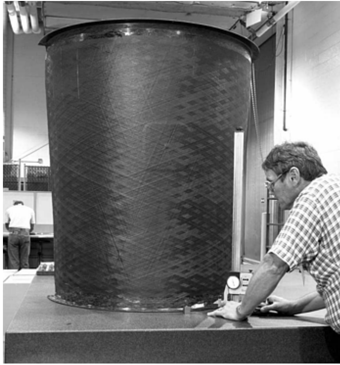
Fig. 19 F110 carbon-PMR filament-wound duct
