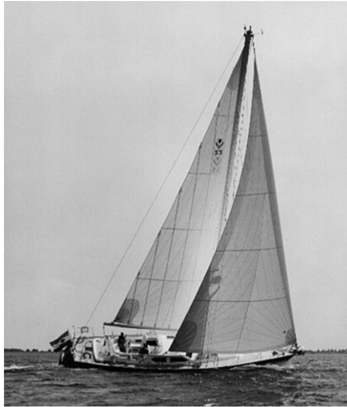
Fig. 3 Contest 55 sailing yacht with hull manufactured by vacuum infusion. Courtesy of Conyplex Shipyard, Medemblik, the Netherlands
