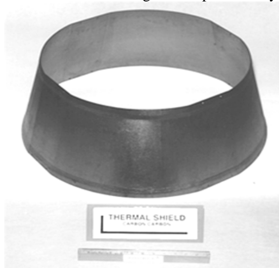
Fig. 6 Uncoated, as-fabricated carbon-carbon thermal shield. Courtesy of Lockheed Martin Astronautics
