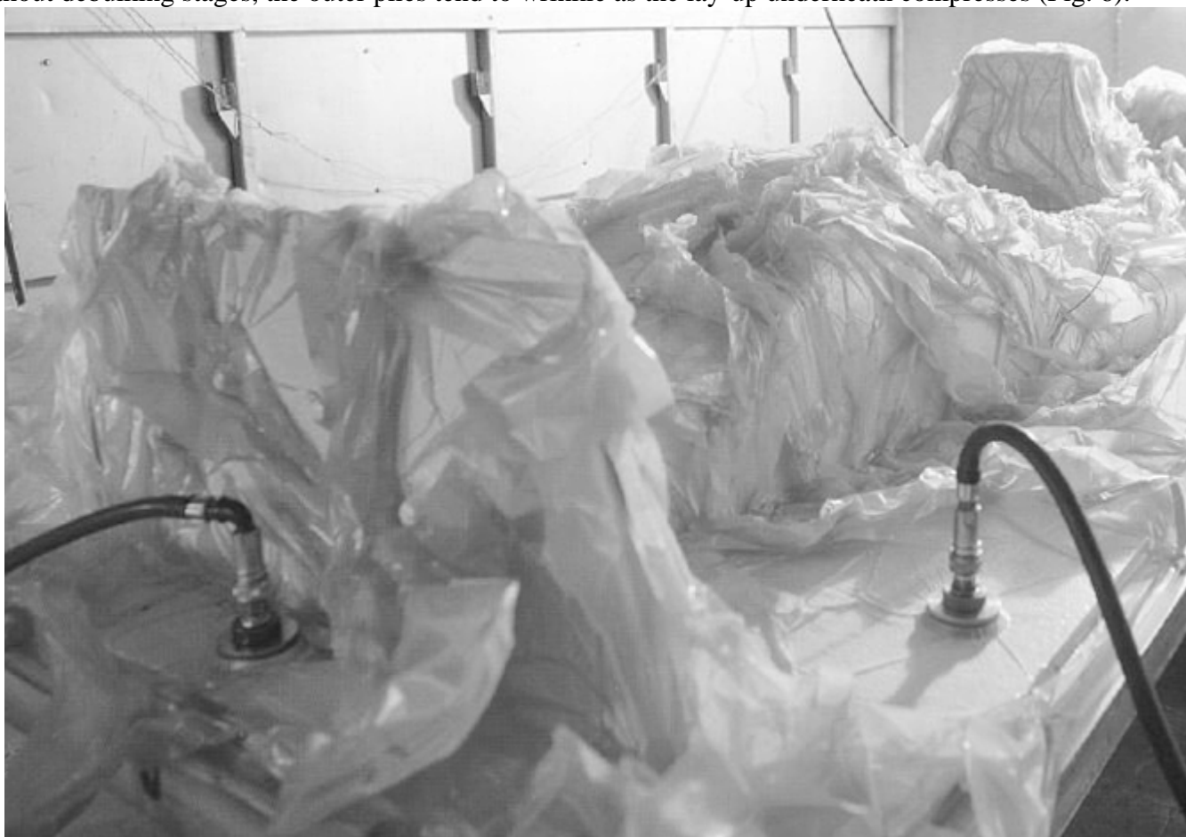
Fig. 6 Debulking of racing car monocoque lay-up. Courtesy of Nigel Macknight, Motorbooks International
