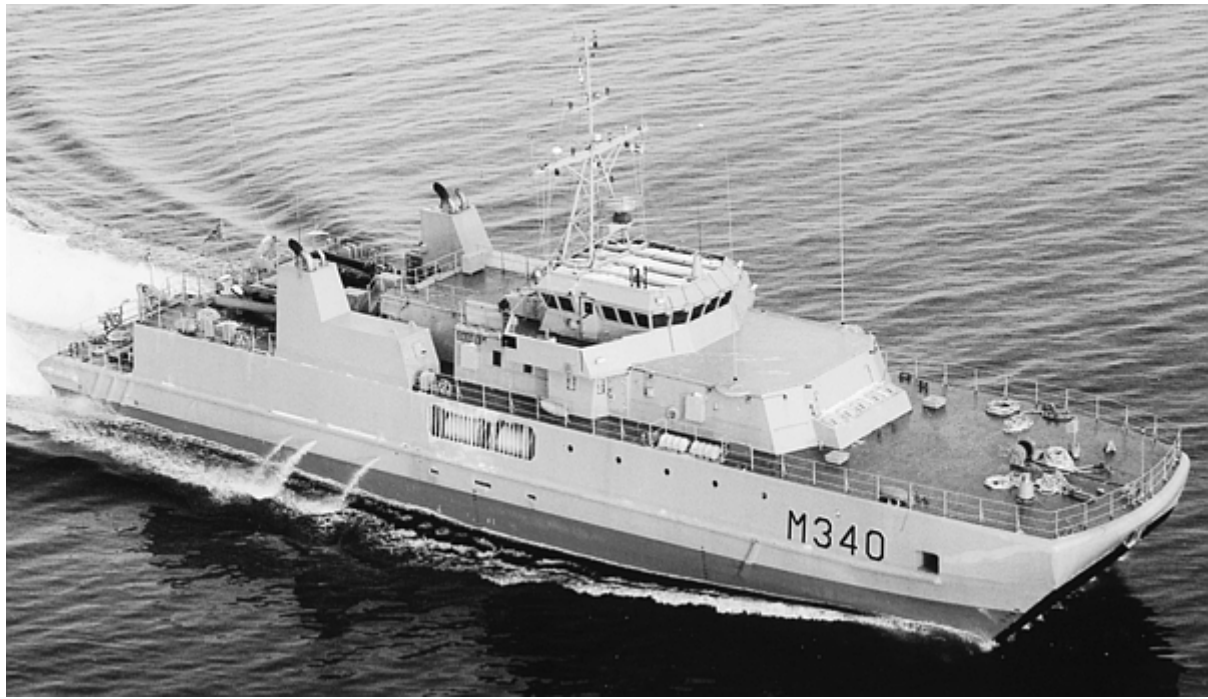
Fig. 4 Open molded composite (sandwich construction) Norwegian Navy mine hunter. Courtesy of Kvæner Mandal
