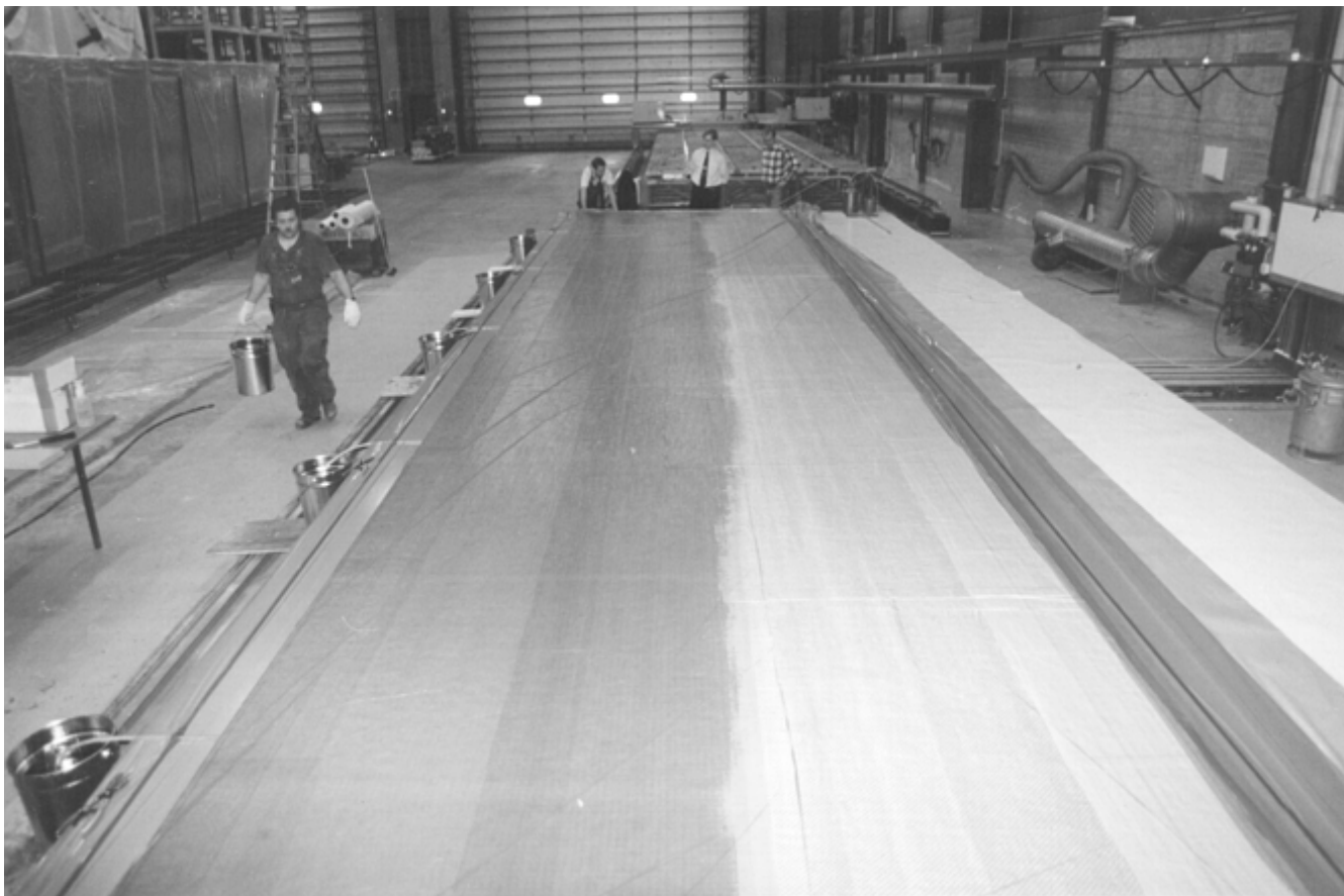
Fig. 6 Vacuum infusion of a 3.2 \times 12 m ( 10.5 \times 39 ft) glass fiber/vinyl ester sandwich illustrating the technique for creating a hull panel for the corvette shown in Fig. 7. Courtesy of Kockums Shipyard, Karlskrona, Sweden
