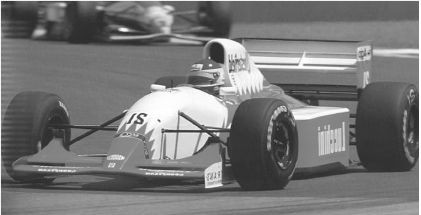
Fig. 8 Lola BMS Ferrari Formula 1 car. All structure, including wings, fairings, and monocoque, is molded by hand lay-up of woven prepreg and autoclave cured. Courtesy of Nigel Macknight, Motorbooks International
