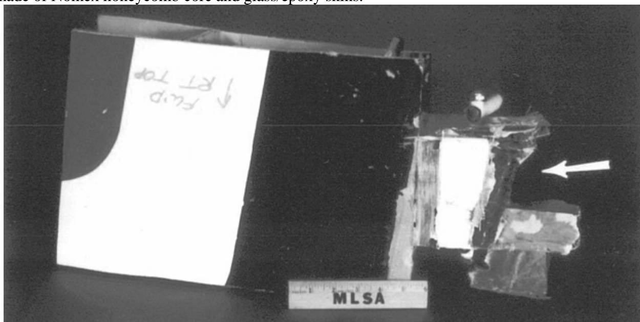
Fig. 8 Section of failed wing spar
