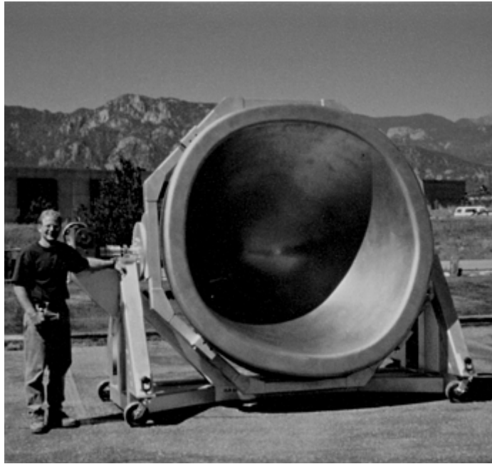
Fig. 2 Autoclave curing mold for aircraft radome
