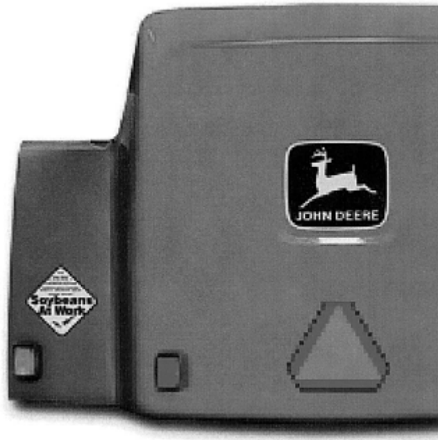
Fig. 1 Harvester part manufactured using soybean-oil- based polymer resin
