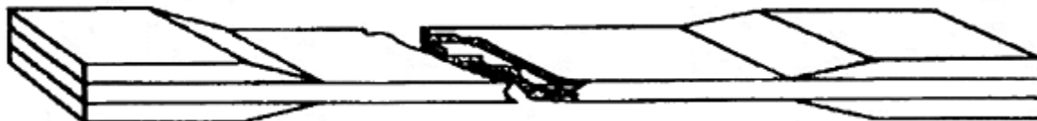
Fig. 1 Typical tension failure of multidirectional laminate using a tabbed coupon
