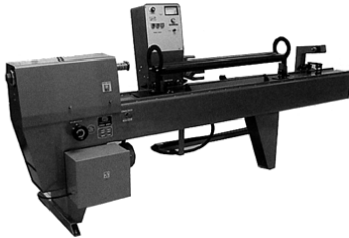
Fig. 6 Automatic shrink tape wrapping machine. Courtesy of Century Design
