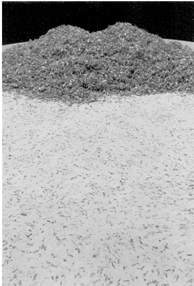
Fig. 44 SMC patio table containing recycling material (with loose recycle shown on top of the table)
