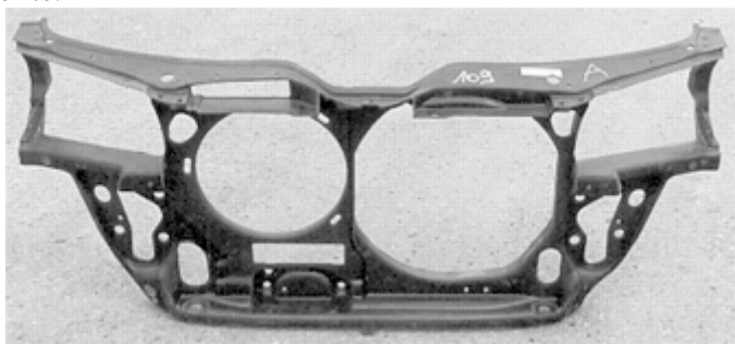
Fig. 37 Technical front end (structural support) for Ford Galaxy and Volkswagen Sharan manufactured by SMC compression molding
