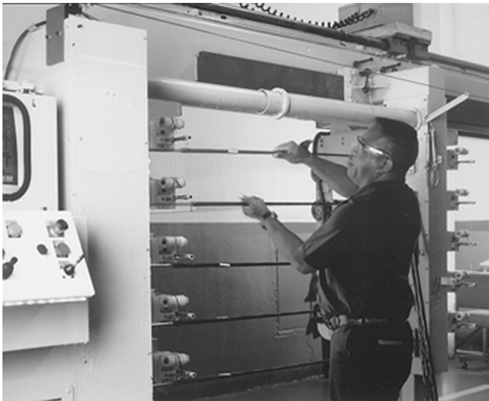
Fig. 8 CNC filament winding of multiple golf shafts. Courtesy of True Temper Sports Company
