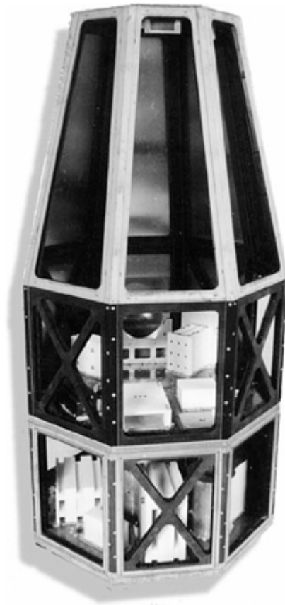
Fig. 3 Composite grid structure for the fast orbit-recording transient events spacecraft. Courtesy of Composite Optics Inc./Los Alamos National Laboratory
