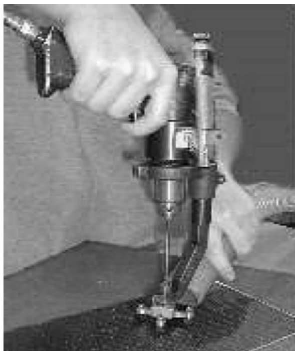
Fig. 3 Hand-feed drill motor with hydraulic dash pot for feed control
