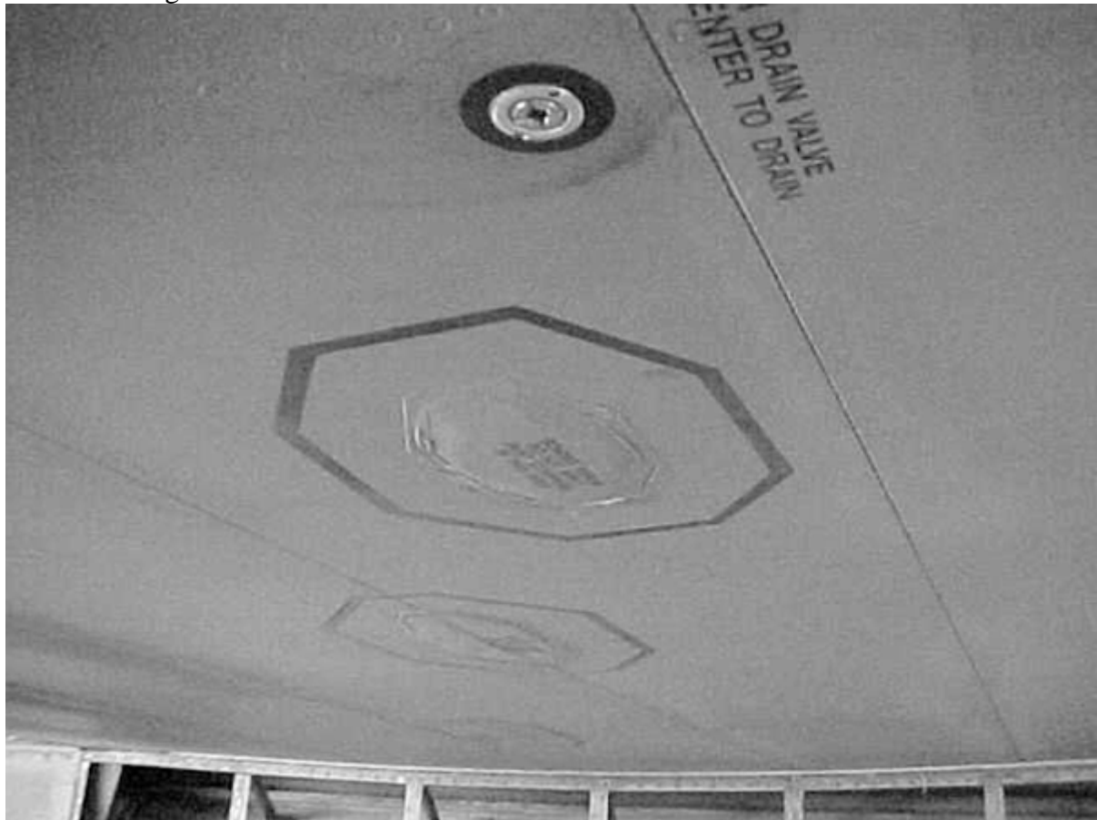
Fig. 6 Doublers installed on C-141 for “weep hole” repair
