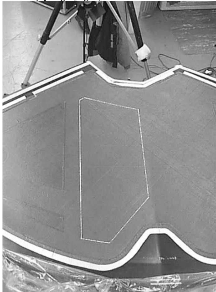
Fig. 5 Laser ply outline projection system in use on aircraft wing and fuselage fairing tool. Courtesy of Assembly Guidance Systems
