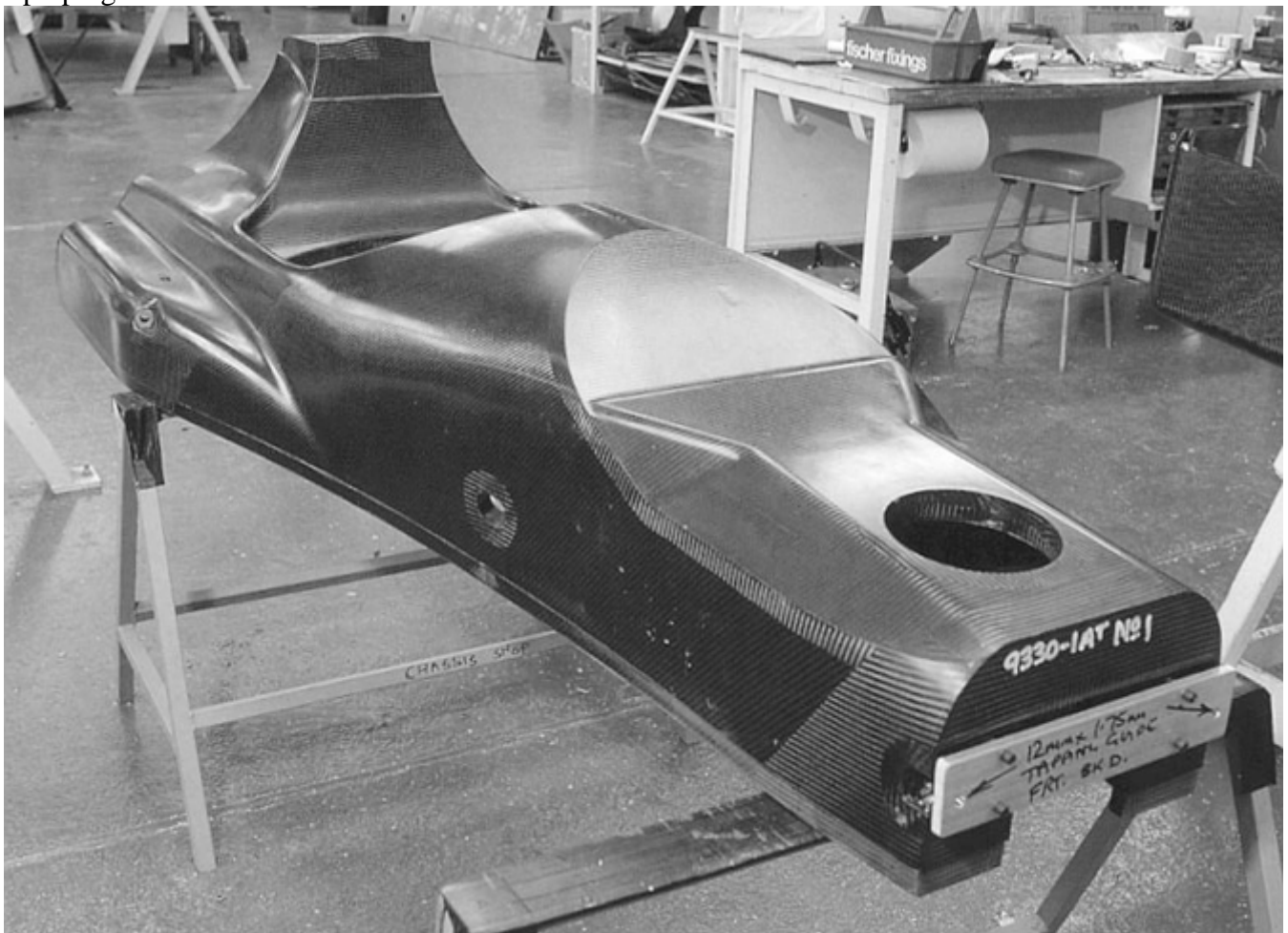
Fig. 7 Autoclave molded Lola Formula 1 car chassis upper half. Courtesy of Nigel Macknight, Motorbooks International
