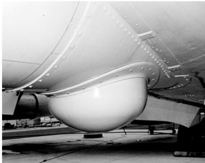
Fig. 5 Quartz/PEKK radome on RC-135 aircraft. Courtesy of Raytheon Systems Co.
