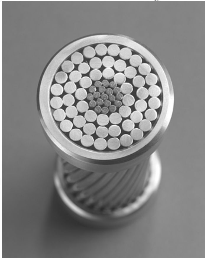
Fig. 8 Cross section of an electrical conductor for power transmission. The core consists of 19 individual wires made from a continuously reinforced aluminum MMC produced by 3M. The MMC core supports the load for the 54 aluminum wires and also carries a significant current, unlike competing steel cores. Courtesy of 3M
