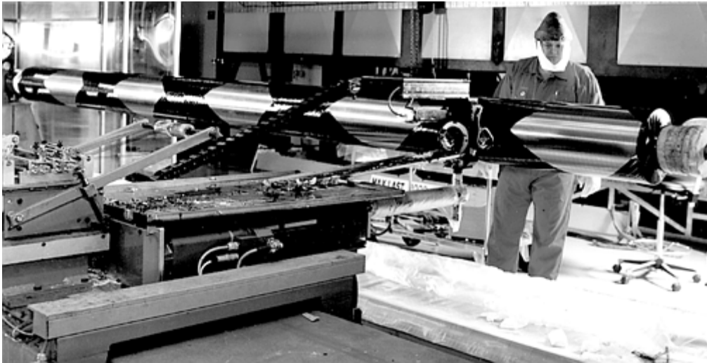
Fig. 18 Commercial roller filament-winding. Courtesy of Applied Composites AB, Celsius Group
