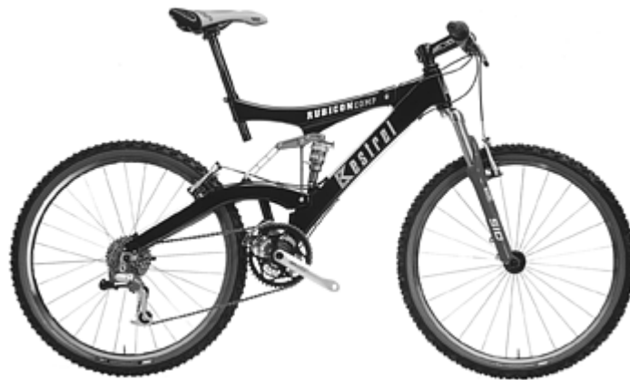
Fig. 1 One-piece carbon/epoxy bicycle frame. Courtesy of Kestrel
