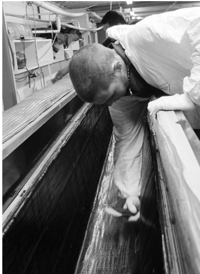
Fig. 12 Laminating a prepreg mast section. Courtesy of Southern Spars
