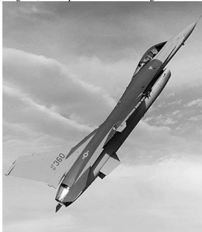
Fig. 2 An F-16 aircraft, illustrating the ventral fins, which are located on the bottom of the fuselage just aft of (behind) the wings. The ventral fins are now assembled from 6092/SiC/17.5p discontinuously-reinforced aluminum sheet material produced via a powder metallurgy process.
