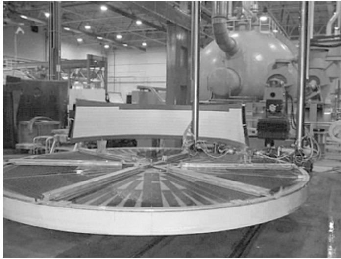
Fig. 5 Automated ultrasonic inspection system with a turntable
