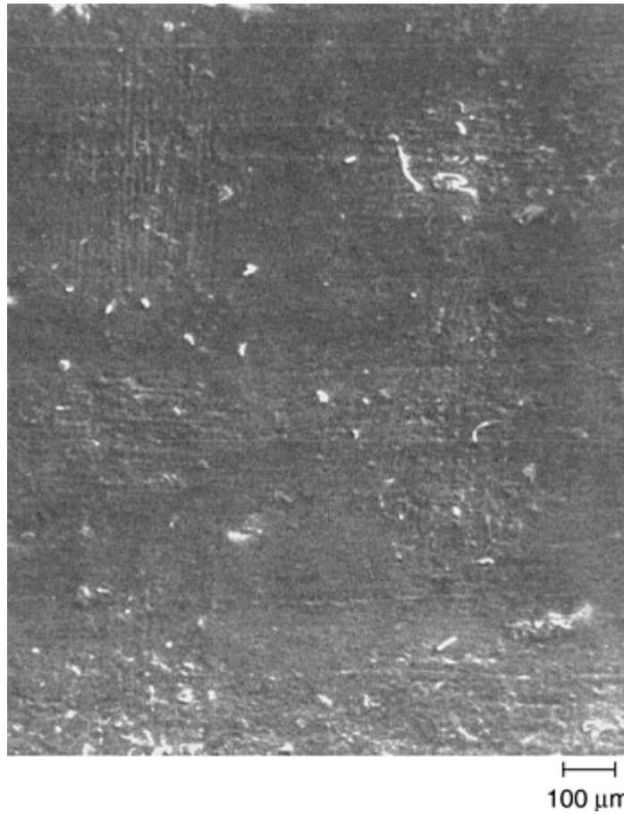
Fig. 2 Low magnification SEM view of shiny areas on Kevlar/epoxy paddle surface. 48×
