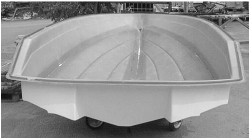
Fig. 5 Vacuum infused 5.1 m (17 ft) boat hull
