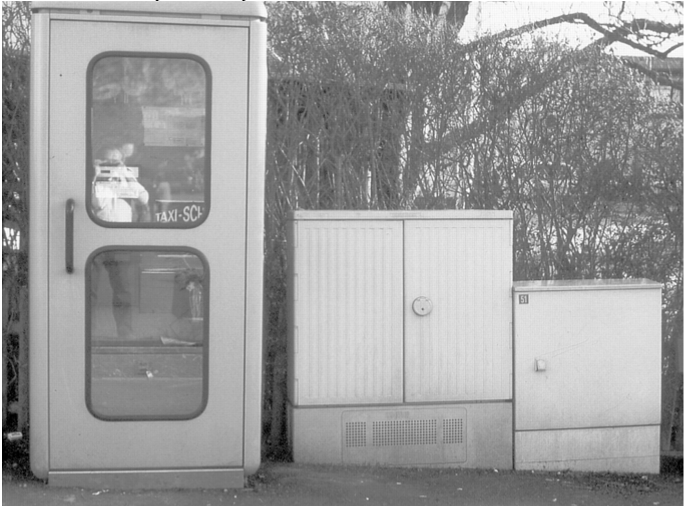
Fig. 32 Unpainted cable and telephone boxes manufactured by SMC compression molding. The boxes, exposed to the weather for 25 years, are shown next to an old painted telephone booth.
