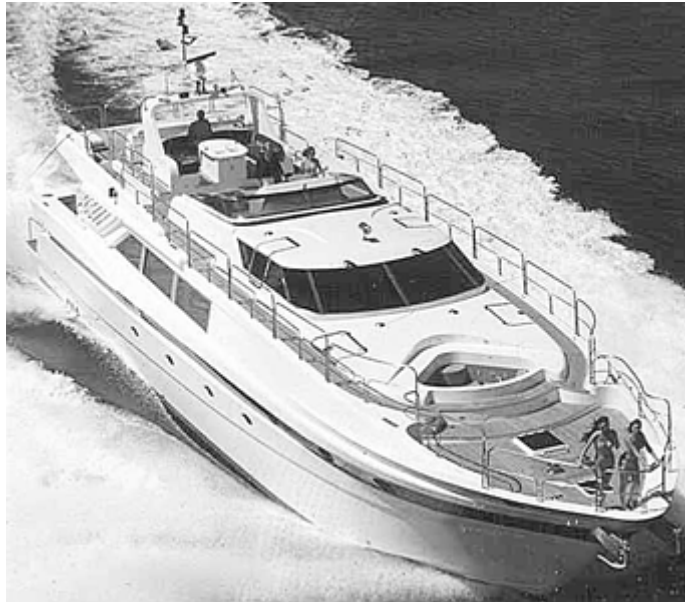
Fig. 2 Open-molded composite boat hull and deck for luxury cruiser. Courtesy of Gulf Craft-UAE
