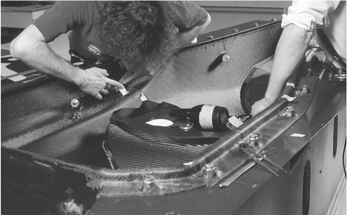
Fig. 4 Lola BMS-Ferrari Formula 1 car monocoque, manufactured by hand lay-up of woven carbon fiber prepreg. Courtesy of Nigel Macknight, Motorbooks International
